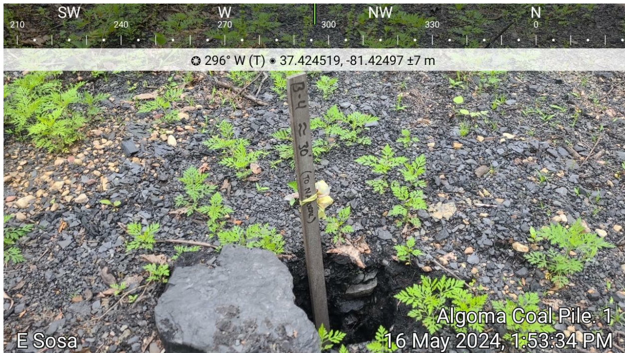
Figure 12-1: Photo of wooden stake and borehole from Marshall Miller (1997) confirming depth to natural ground (top is facing direction, Lat/Long, and including date)
